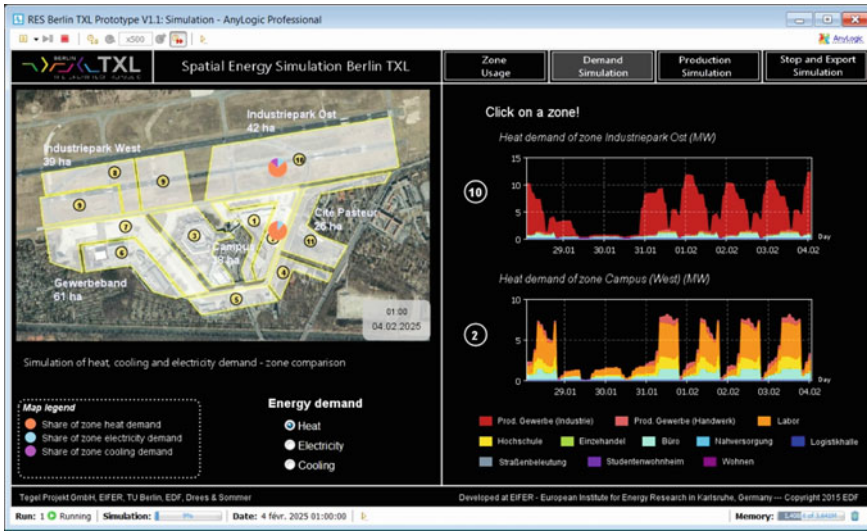
Fig. 5 User interface simulation: calculation of the hourly heat demand in selected construction zones
