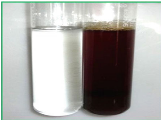
Fig. 1 Solutions of ZnO before ( left ) and after ( right ) exposure to the culture supernatant of S. thalophilum
