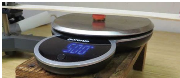
Fig. 7 Pressing on the hydrogel pearl being put on the scale
