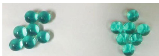
Fig. 4 Hydrogel pearls after 6 h in warm water ( left ) and cold water ( right )
