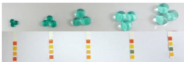
Fig. 5 Hydrogel pearls after 6 h in vinegar solutions, pH grows from the left to the right hand side
