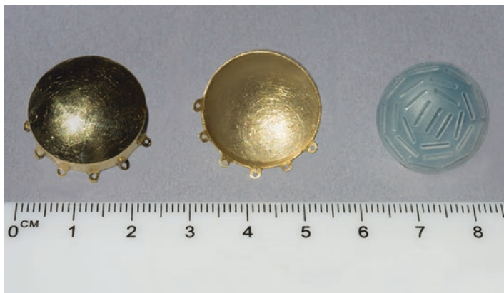
FIG. 8.4. Picture of a 20 mm plaque. Top view of the gold plated plaque ( left ); plaque inverted showing the side in contact with the sclera ( center ); Silastic seed carrier insert ( right )
