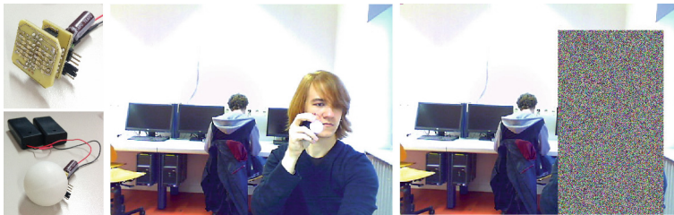
Fig. 3. A first proof-of-concept implementation of the DCI as opt-out: only regions surrounding a detected infrared beacon are anonymised.
