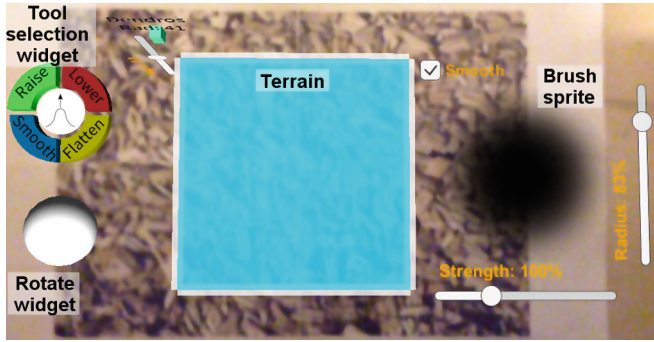
Fig. 3. Snapshot of the UI of the DEM editor. The terrain mesh, tool selection widget and brush sprite are indicated.
