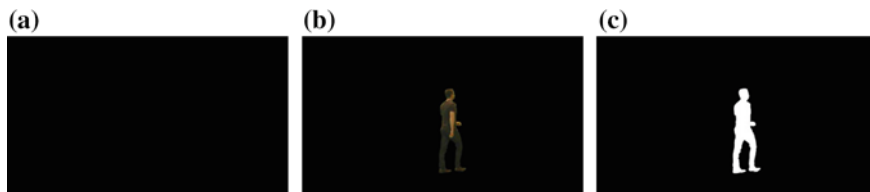
Fig. 2 a Background model, b current frame, c foreground object obtained from (a, b)
