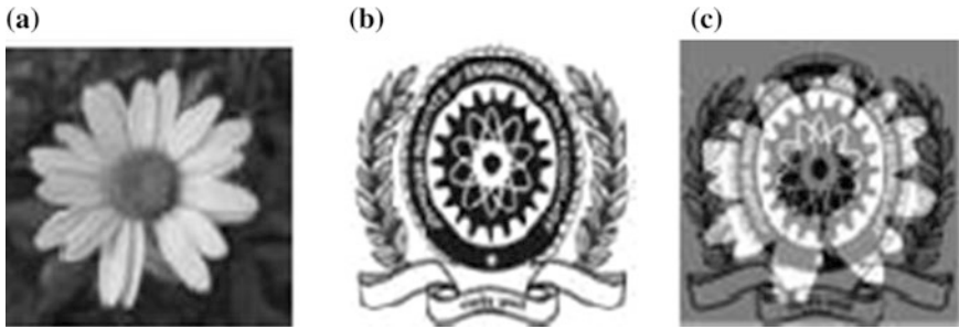
Fig. 4 LSB results. a Original, b watermark, and c watermarked images (visible watermarking)
