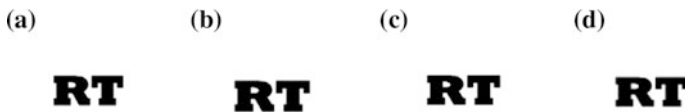
Fig. 4 Extracted watermark from various test images. a NCC = 0.993, b NCC = 0.991, c NCC = 0.996, d NCC = 0.995
