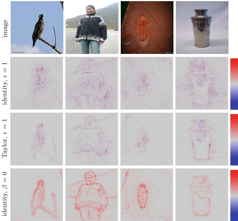
Fig. 3. Top row shows original unwarped image. Remaining rows show heatmaps produced by various parameters of the LRP method.
