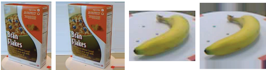
Fig. 2. Border replication for squaring dataset images. The outer pixels of the longer side are replicated along the axis of the shorter side until the entire image is quadratic.
