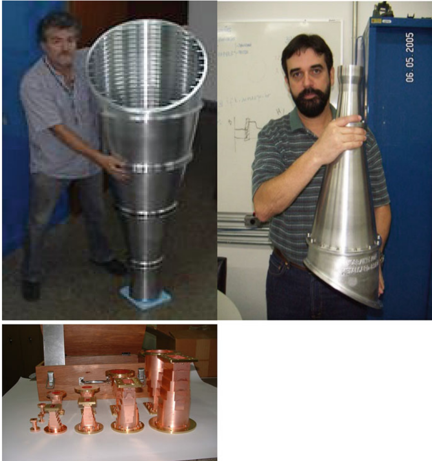
Fig. 15 Horns (a, b) and transitions (c) provided by INPE for the ARCADE 2 experiment
