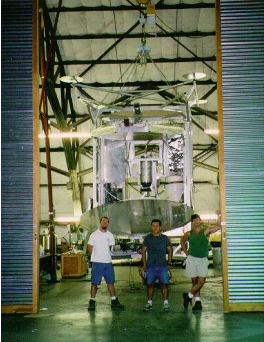
Fig. 8 BEAST experiment before flight showing the 2.6-m diameter flat mirror
