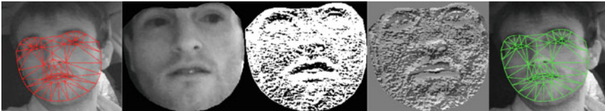
Fig. 3 From left to right: Input image with initial guess for the shape model (1) warped onto the base mesh (2) and transformed by the MCT (3). Image (4) shows the difference image \mathbf{r}(\mathbf{p}) which is used to calculate the optimized parameters. The result of the iteration step for matching the MCT AAM onto the face is shown in the last image (5)
