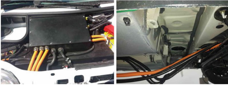
Fig. 7 Battery pack in demonstrator vehicle ( left front, right rear )
