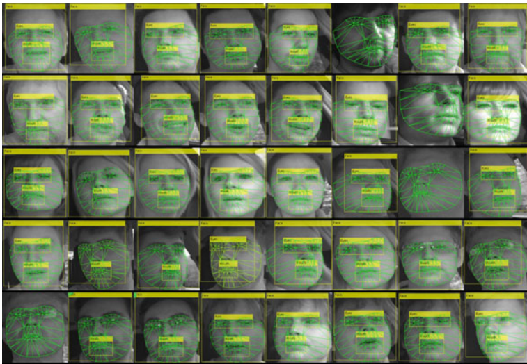
Fig. 9 Examples for matching results of the MCT AAM on different previously unseen faces with different head-poses. The MCT AAM returns good results even though some parts are occluded by beard growth, hair or glasses
