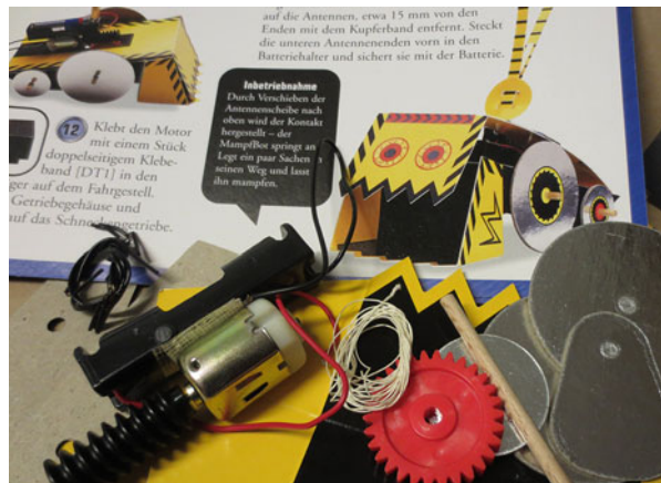
Fig. 11 Components of a battery-driven construction kit with cardboard, wood, and electrical motor
