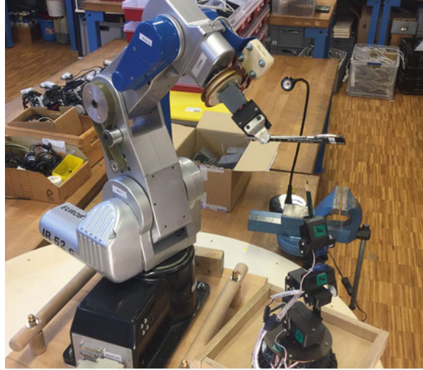
Fig. 9 Two small and flexible multi-axis robots for educational use. The large one is factory made, the other one a programmable assembly kit
