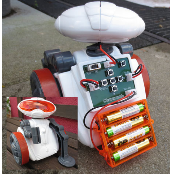
Fig. 5 The Galileo-Roboter as a nice example for a programmable assembly kit. All moves are embedded in not changeable hardware and may be coded via step by step on surface
