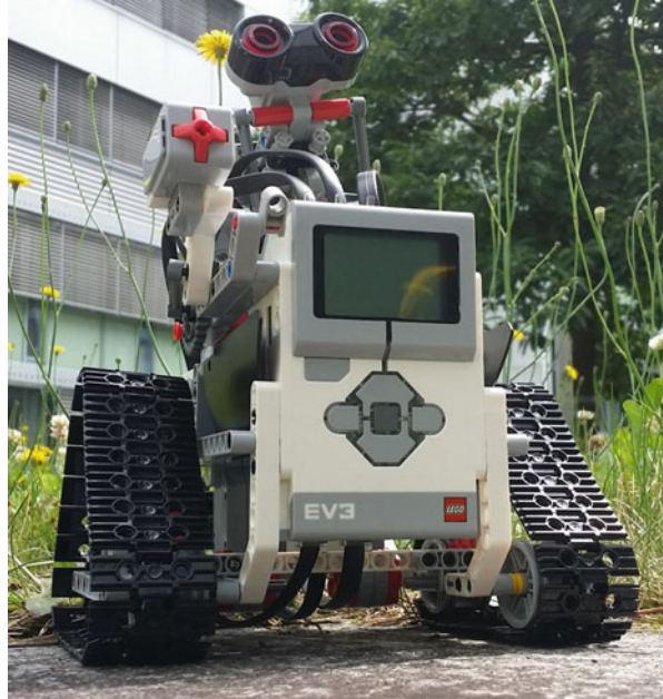
Fig. 2 Common edutainment robot on caterpillars. It should be programmed via surface or PC using proprietary (icon-based) or nonproprietary software
