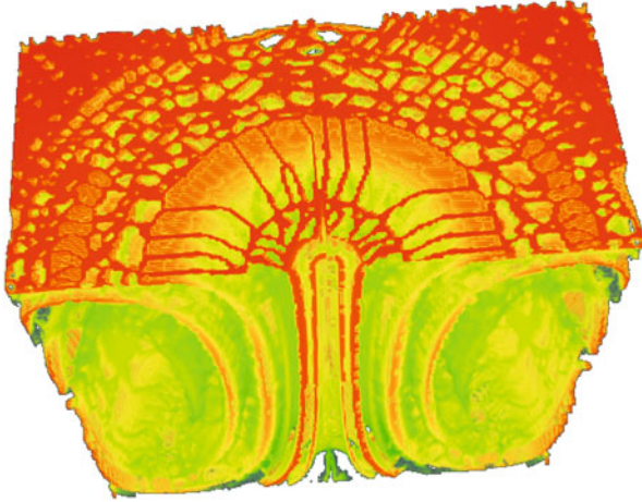
Fig. 1 Oversegmentation of the LCS of a simple convection cell flow due to variation and noise in the FTLE field
