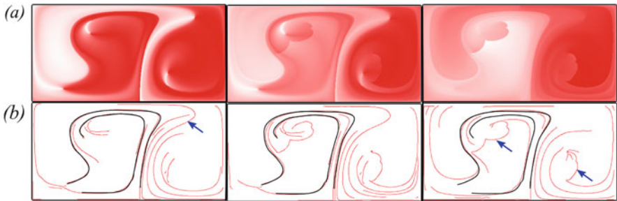
Fig. 8 Illustration of weighted combination of \Phi and avgDir field. (a) Combined attribute field; (b) edges detected from the super field. The dark gray curves on top are stable edges that do not change with weights. The weights of \Phi and avgDir from left to right are \alpha_1 = 0.1, \alpha_2 = 0.9 ; \alpha_1 = 0.5, \alpha_2 = 0.5 ; \alpha_1 = 0.9, \alpha_2 = 0.1 , respectively. The parameters of Canny edge detector are \sigma = 1.0, \alpha = 0.3, \beta = 0.8
