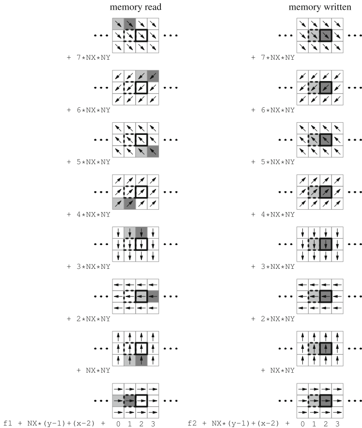
Fig. 13.2 Diagram showing the memory locations read ( left ) and written ( right ) during the updating of two consecutive nodes when the populations f_i(x, y) are stored at the linear indices NX \cdot (NY \cdot d + y) + x . The data for the node at (x - 1, y) is outlined with a dashed line , and a thick outline shows the data for the node at (x, y)
