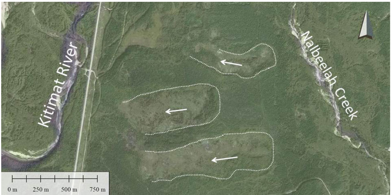
Fig. 25.9 Wetland-filled earth flows at Nalbeelah Creek (sites 12–14; Fig. 25.7). British Columbia Ministry of Forests, Lands, and Natural Resource Operations imagery
