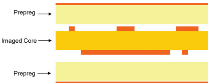
Fig. 11.9 Schematic of the multilayer lamination process
