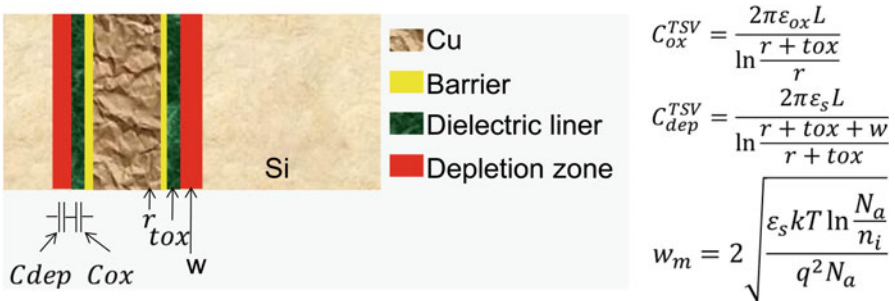
Fig. 5.2 Schematic drawing of TSV capacitance
