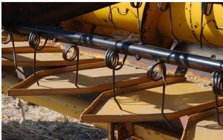
Fig. 22.1 Particular of the triangular plates applied at the head for wheat
