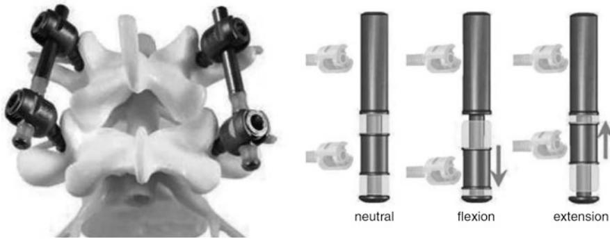
Fig. 16 NFlex device in neutral, flexion and extension positions. (Source: https://www.ncbi.nlm.nih.gov/pmc/articles/PMC3424174/ )
