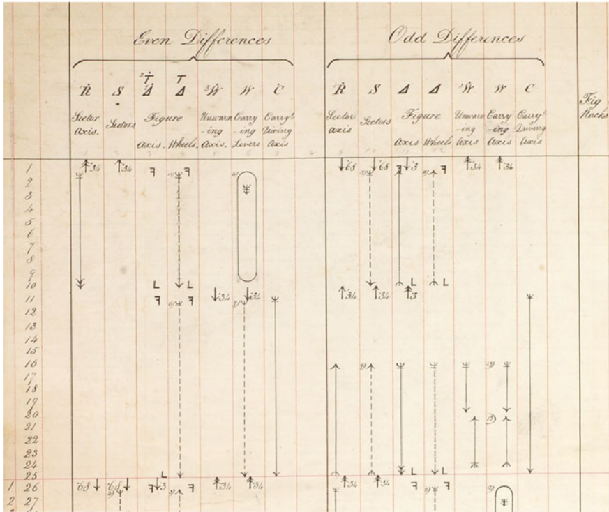
Fig. 33.3 Mechanical Notation: Cycle for addition and carriage in Difference Engine No. 2 (part). Credits Science Museum/Science and Society Picture Library
