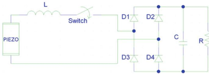
**Fig. 5** The general “Series SSHI” circuit schema
