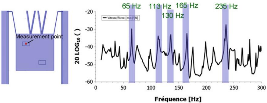
**Fig. 12** Frequency response of the mechanical system
