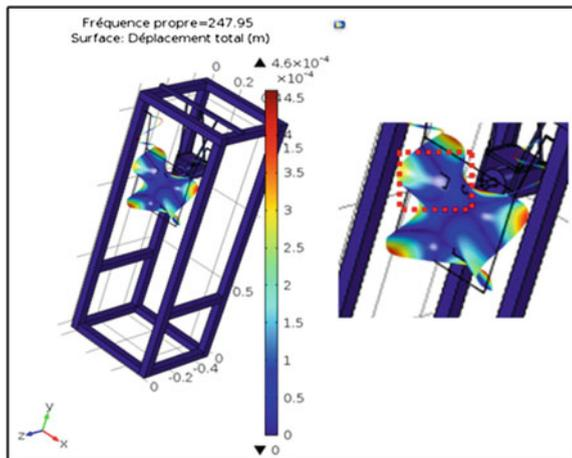
The Fig. 15 proves the deformation of the left piezoelectric element used to damp the mechanical vibrations. Moreover, for this frequency, the left piezoelectric element is placed next to the vibrations wave anti-node; thus, the maximum efficiency of damping is achieved.
