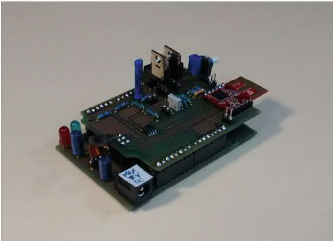
**Fig. 7** Picture of the designed WSN node for AVC system
