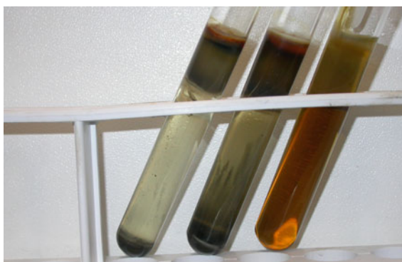
Fig. 6.5 Cultures of active IRB, the two test tubes on the left show positive ferric iron reducing culture in different cell concentrations, the last tube on the right shows negative ferric iron reducing culture. (Courtesy of Extrin Consultants)
