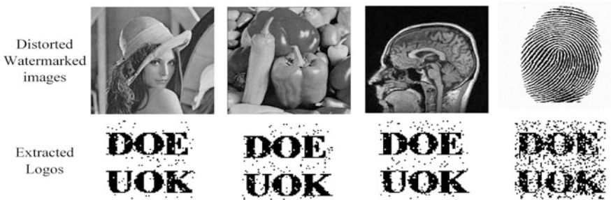
Fig. 14 Distorted watermarked gray scale images by Gaussian noise and extracted Logos (Variance 0.001)
