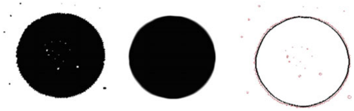
Fig. 6 Left the circle object with a noise with high curvature and an unsmooth boundary. Middle the object smoothed by (15). Right isolines representing the boundaries of the original (red) and of the smoothed objects. The boundary slightly shrinks. We used method [2] working on a regular grid
