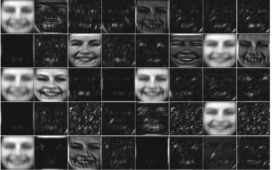
Fig. 2. Magnitude response of Gabor filter with 8 orientations and 5 dimensions. Image corresponding to subject F06 from KDEF database [33].
