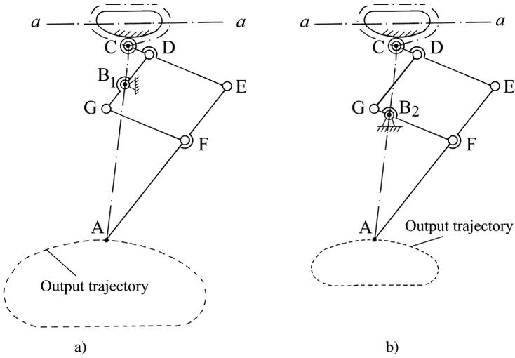
**Fig. 2** Leg mechanism with two output trajectories
