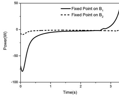
**Fig. 5** Power consumption of input motion during leg's swing phase when fixed point on  $B_1$  and  $B_2$
