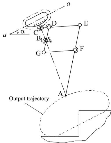
allows one to change the orientation of the input trajectory. Such an adjustment allows the walking robot to climb stairs.
