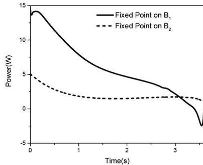
**Fig. 6** Power consumption of input motion during leg’s stand phase when fixed point on  $B_1$  and  $B_2$
