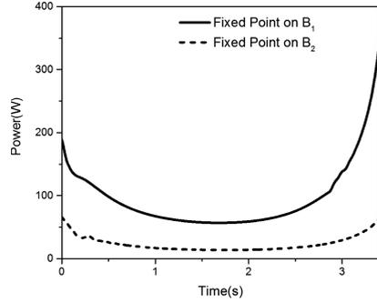
**Fig. 7** Power consumption of input motion during leg’s swing phase when fixed point on  $B_1$  and  $B_2$
