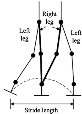
stable propelling of the body. The curved segment is related to the non-propelling phase, which is produced by leg when it swings from back to forth [18].
