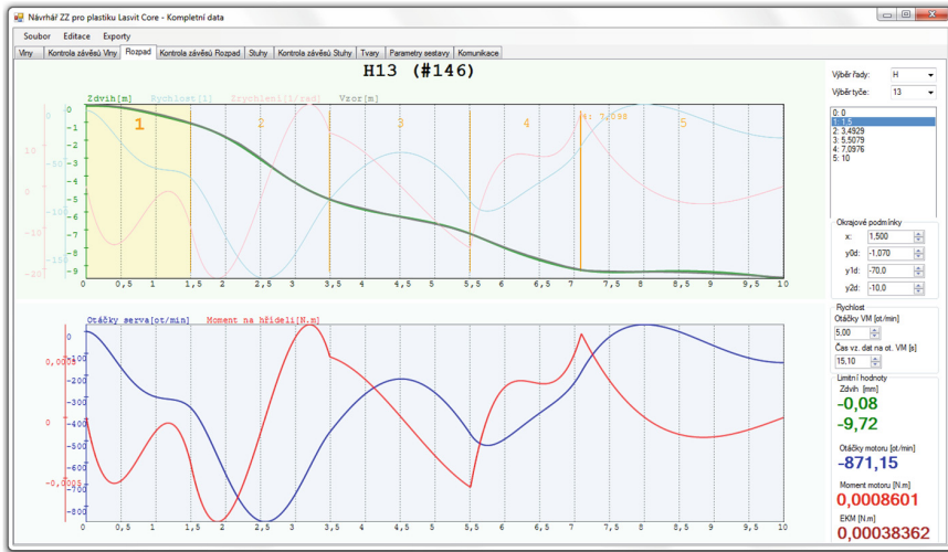
Fig. 5 Practical demonstration creating of displacement diagram (green stroke, blue motor speed, red motor shaft torque) (Color figure online)
