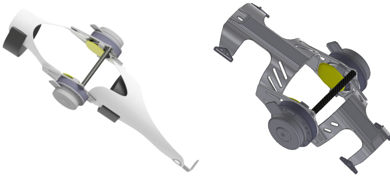
Fig. 4 Robotic orthosis composite and metallic variant
