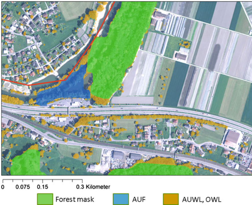
Fig. 4.4 Example of a true color orthoimage with the forest mask based on the FAO definition, estimated AUF, and AUWL and OWL (From Vidal et al. 2016)
