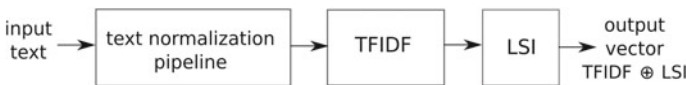
Fig. 1 Generic treatment of input text to obtain input vectors used in our algorithms
