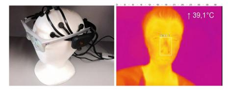
**Fig. 3** EEG device example—Emotiv Epoc (on the *left side*) and the thermal image example with area for measuring the temperature set around the nose of the participant (on the *right side*)
