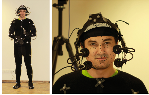
Fig. 1. The marker setups for the optical mocap systems. On the left: body mocap consisting of 53 14 mm retroreflective markers for the VICON system, on the right: 54 black passive markers for the VICON Cara system.
