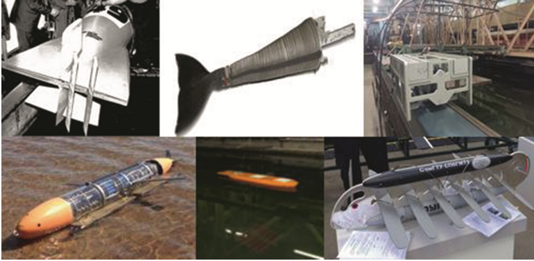
Fig. 1. Underwater vehicle «Aphalina» with flapping wing propulsor [3], bionic propulsor of underwater robot [4], small-sized inspection ROV [5], SMTU underwater glider [6], SMTU scaled mock-up of wave glider [7], SamGTU-SMTU wave glider (underwater module)
