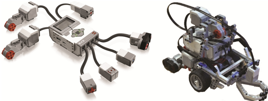
Fig. 3. Lego® Mindstorms EV3 Education kit and mobile robot constructed from the kit
