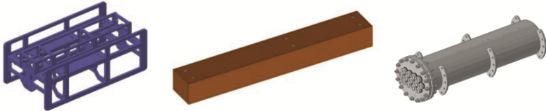
Fig. 3. The hull components: frame, element providing neutral buoyancy and pressure hull for the equipment
