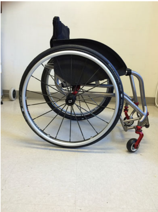
Fig. 22.1 Ultra-lightweight wheelchair that allows adjustment of rear wheel position
