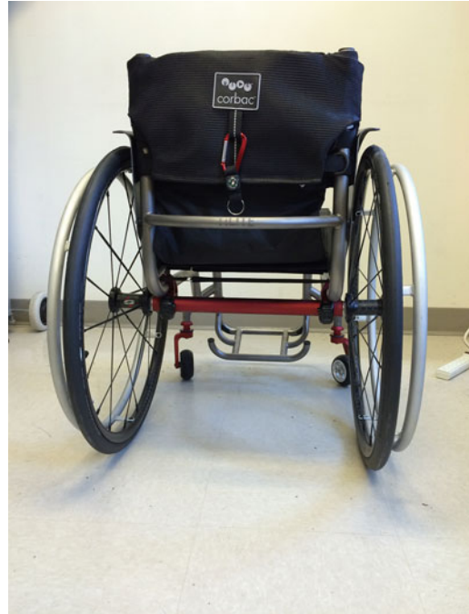
Fig. 22.2 Ultra-lightweight wheelchair showing camber, where the distance between the base of the wheels is wider than the top
