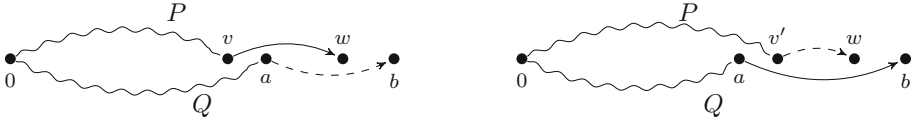
Fig. 3. Computation of T[w, (a, b)] . Either a path P = (0, \dots, w) ends with an edge (v, w) with v \leq a (left) or it ends in an edge (v', w) with v' > a (right).
