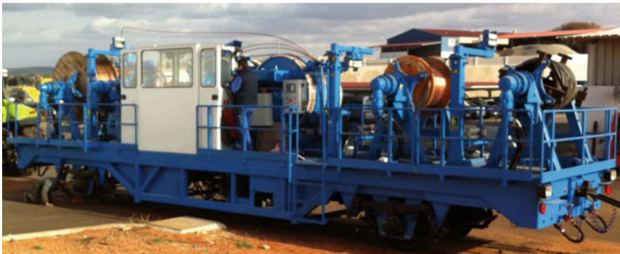
Fig. 1 Train with braking machine and cable coils
