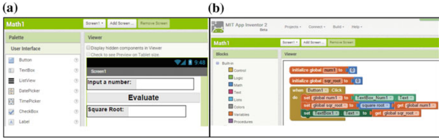
Fig. 1 MITApp12 example: toy application to evaluate the square root of a user inputted number. Application user interface design and programming. a User interface design. b Blocks programming
