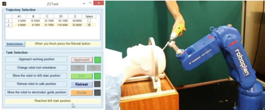
Fig. 8 Performing assisted drilling, with orientation- and depth-control
