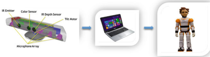
Fig. 1 Experimental set-up: Kinect , computer and ZECA
