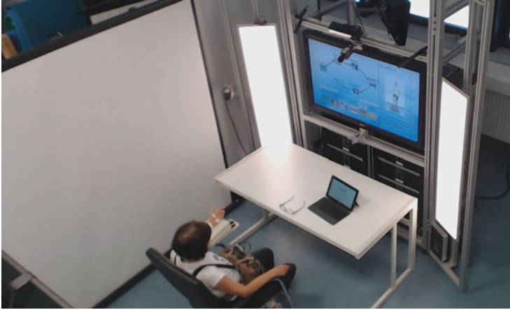
Fig. 1.7 Multi-sensorial setup of a data recording where a user interacts with a Companion -system
