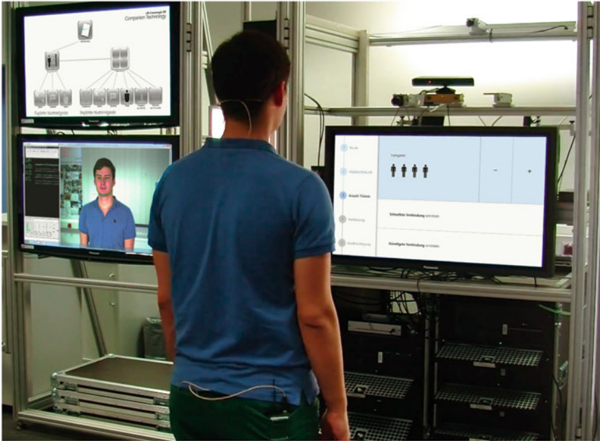
Fig. 25.1 A user interacting with the ticket purchase system. While the application is shown on the right screen in front of the user, the left screens visualize internal system states and signal processing details. Various sensors can be seen mounted on the rack
