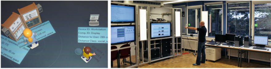
Fig. 10.2 Emulation by tangible interaction ( left ) and later real situation with various sensors ( right ). Moving the toy figures on the table results in almost equal signals as the person tracking via laser range finders as described in [18]
