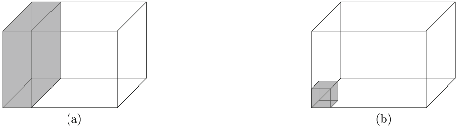
Fig. 3. The two splitting modes of 3D-NRRP. In both cases, the gray polyhedra is attributed to \{v_1, \dots, v_{k-1}\} , the white one to \{v_k, \dots, v_n\} .
