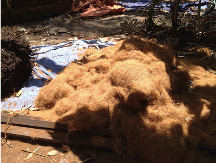
Fig. 20.5 Extracted coir fibers, the raw material for coir products such as geotextiles, © David 2014
