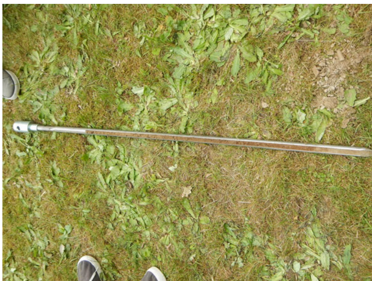
Fig. 5.3 RIDEX soil probe with the soil sample (Source: Karvánková, photo archive 2014)
