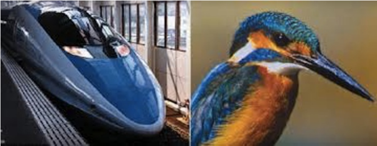
Fig. 7.5 Design of Shinkansen bullet train's nose to decrease noise, inspired by the Kingfisher's beak.
