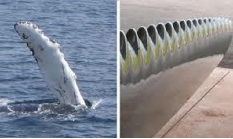
Fig. 7.4 Design of wind turbine blades to increase efficiency, inspired by the tubercles on humpback whale flippers.
