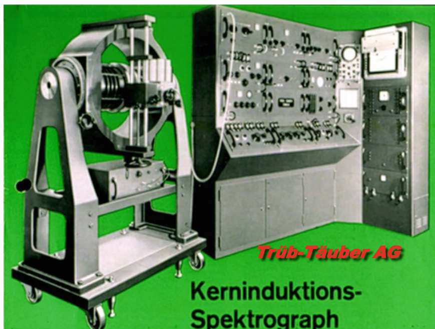
Fig. 8 Commercial NMR spectrometer designed by Primas and built and commercialized by the company Trüb-Täuber AG in Zurich
