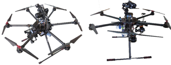
Fig. 10. Prototype of the hexarotor
