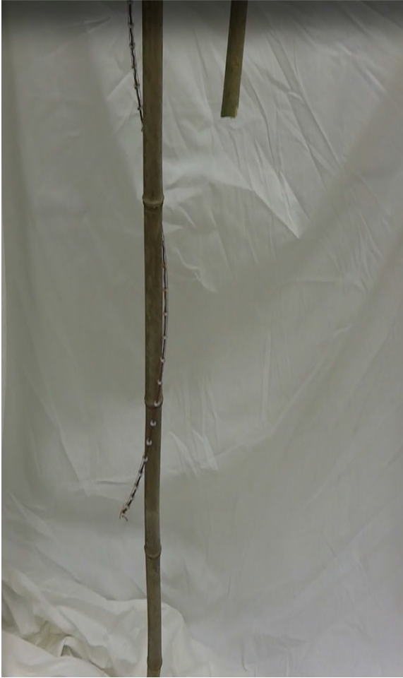
Fig. 3. Tendril robot coiling around bamboo post following circumnutation.
