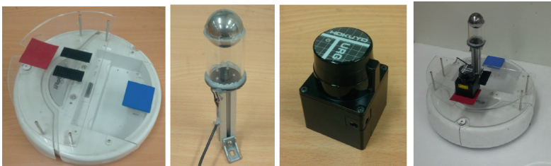
Fig. 1. Mobile robot (a) i-Robot ROOMBA mobile (b) omnidirectional camera ( 640 \times 480 pixels) (c) HOKUYO laser sensor measurement part ( 240^\circ measuring area with 0.36^\circ resolution) (d) mobile robot mounted with sensors
