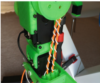
(a) 2 composite tendons on the biceps servo pulley.
