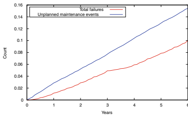
(a) Number of compressor failures and unplanned maintenance events over time. Note that each failure also causes unplanned maintenance, but these are not included here.
