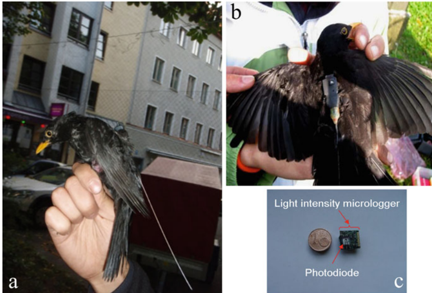
Fig. 13.3 Bird tagging. (a, b) Blackbirds were tag using a “backpack”. This consisted of two devices, a light logger and radio-transmitter, stuck together using shrinking tubes and then attached to the animal with rub and cotton harnesses pulled through the legs. (c) Light logger (Sigma Delta Technologies, Australia). The loggers weighed 2.4 g and were composed of an electric circuit linked to a photodiode, whose spectral responsivity ranged from 300 to 1100 nm, with a peak around 780 nm. They recorded and stored light intensity every 2 min for the entire time. We calibrated the loggers against a photometer (LI-1400 and LI-2100, LI-COR, USA) in order to convert frequency into lux (illuminance) and watt/m 2 (irradiance) values
