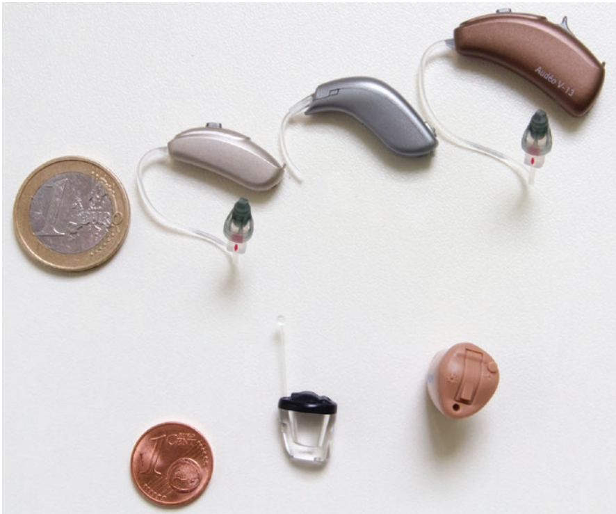
Fig. 4.12 Different types of hearing aids. Hearing aids may be placed behind the ear – top , three examples, or in the ear canal – bottom , two examples. Depending on individual amplification required, technical setup of sound transmission to the middle ear varies widely (From Neuroth AG, Austria)
