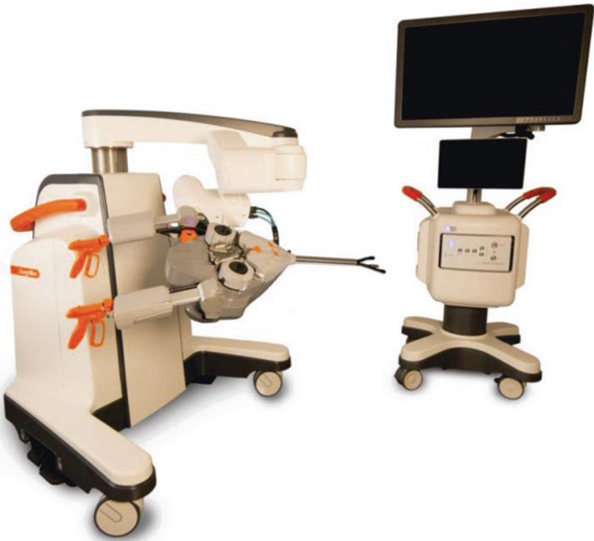
Fig. 21.3 SurgiBot™ Bedside cart and vision console
