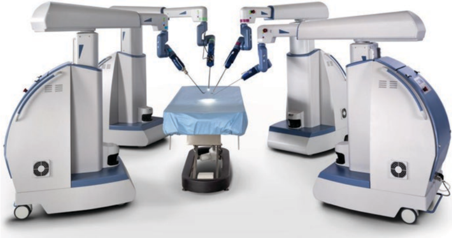
Fig. 21.6 Telelap ALF-X bedside robotic carts
