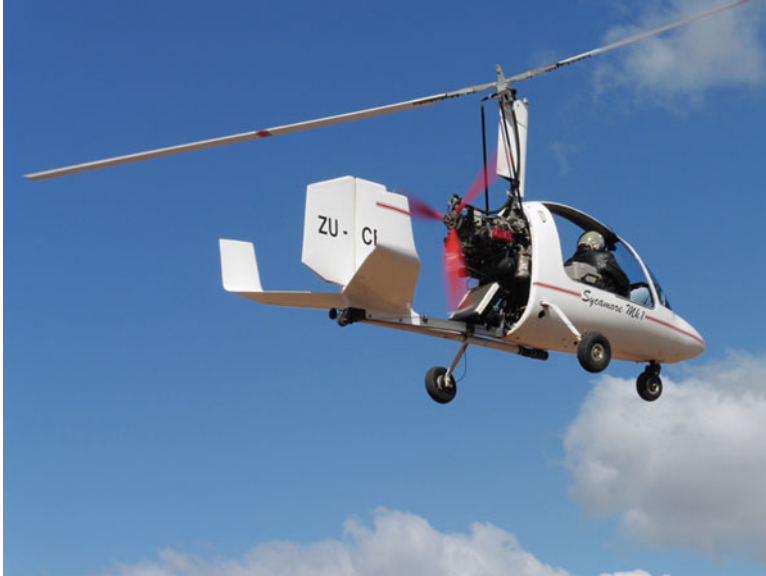
Fig. 19.6 Gyroplane used in pilot aerial releases of sterile male C. capitata . The insulated box of pre-chilled flies is visible behind the pilot, as is the venturi release tube below the fuselage
